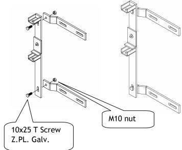
When the gate hangs on an end partition, bolt the fitting to the partition with the accompanying bolts and nuts.
