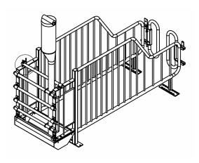
Drill a hole 9 mm in diameter for the drill clamp. Fix this to the water pipe. Note:
