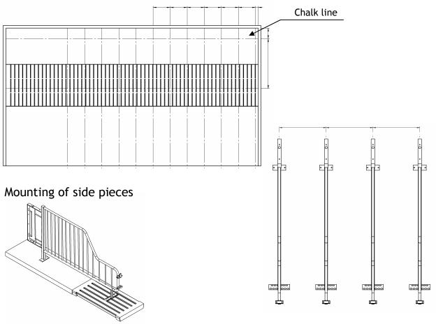
Bolt the outer side piece loosely to the floor. Place the next side piece at a distance of 65 cm measured
