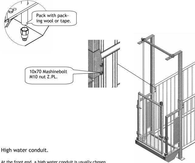
At the front end, a high water conduit is usually chosen. Use post extensions of 106.5 cm to achieve a pipe height of 216 cm. Mount the post extensions as shown on the drawing.
