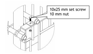
The pipes are fixed with 1" pipeholders, 10x25 mm set screws and 10 mm nuts. Remember to fit plastic plugs at the ends of the pipes.
